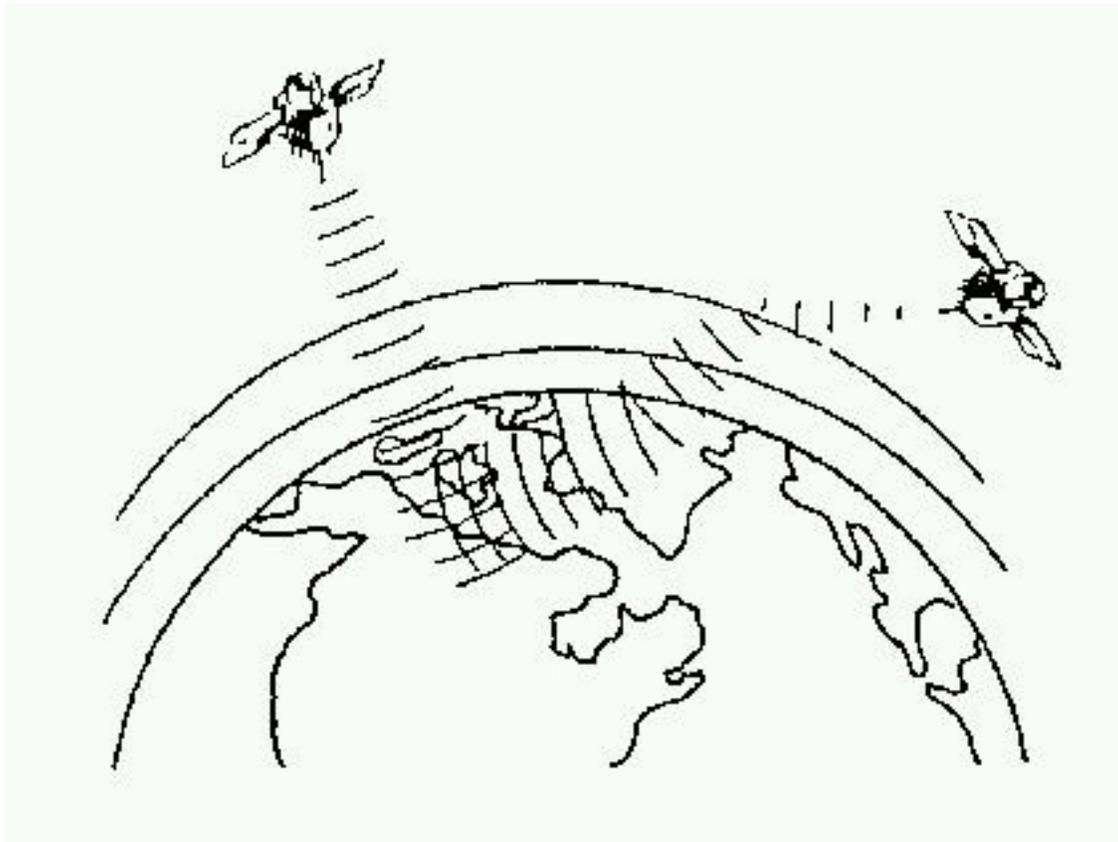
**Figure 1.** Depiction of ionospheric scintillation affect on GPS satellite transmissions.
